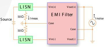
Figure B: Common-Mode Current Attenuation, Imeas / Inoise
