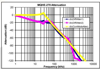
Figure 1: Simulation of calculated common-mode and differential-mode current attenuation. The curves plot the ratio of noise current in a  $50\Omega$  LISN sensing port connected to the noise output side of the filter to the noise current on the input side. The filter case is also connected to chassis ground. Refer to Figures A and B.
