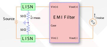
Figure A: Differential-Mode Current Attenuation, Imeas / Inoise
