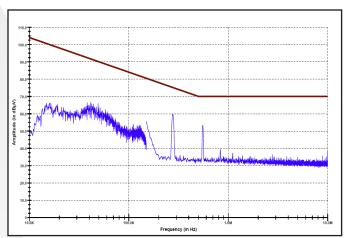
Figure 4: MIL-STD-461E Method CE102 High Frequency Conducted Emissions of the MQME-270-P filter with a MQFL-270-05S at 120W output. Limit line (in brown) is the 'Basic Curve'.
