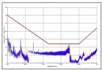
Figure 6: MIL-STD-461E Method RE102 High Frequency Radiated Emissions of the MQME-270-P filter with a MQFL-270-05S at 120W output. Limit line (in brown) is the 'Submarine External to Pressure Hull Curve'.
