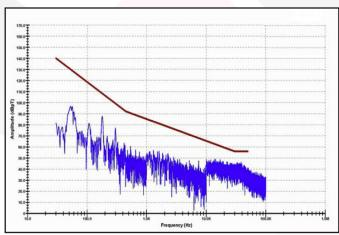
Figure 5: MIL-STD-461E Method RE101 Low Frequency Radiated Emissions of the MQME-270-P filter with a MQFL-270-05S at 120W output. Limit line (in brown) is the 'Standard Curve' from MIL-STD-461C Method RE01, which is more strict than all RE101 limits.
