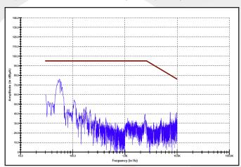
Figure 3: MIL-STD-461E Method CE101 Low Frequency Conducted Emissions of the MQME-270-P filter with a MQFL-270-05S at 120W output. Limit line (in brown) is the 'Submarine Applications DC Curve'.
