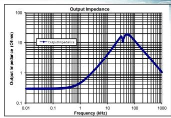
Figure 2: Calculated Output Impedance (magnitude) of the filter looking back into its output pins with the input pins connected to a source with zero source impedance assuming no other parasitic coupling in the system.
